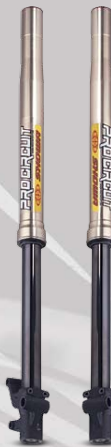
CRF150R Works Showa Suspension
