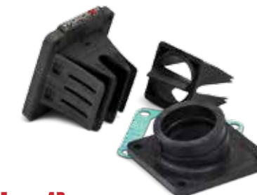
VForce 4R 2019 YZ65/YZ85 Moto Tassinari's VForce4R reed valve system is designed with a shallower petal angle which allows them to open further and with much less force than that of the stock reed system equating to better fuel flow and ultimately more power.
