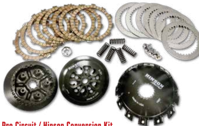
Pro Circuit / Hinson Conversion Kit This kit converts your clutch to a 5 coil spring clutch to help improve clutch performance, and allows the clutch assembly to spin truer creating less heat when the clutch is disengaged and providing a more positive smooth clutch engagement. Includes Clutch Basket, Inner Hub, Pressure Plate, Fiber & Steel Plates, and 5 Hi-Temp Coil Springs. Hinson Clutches are championship proven by almost every major factory team in the world, including Team Monster Energy Pro Circuit Kawasaki.
